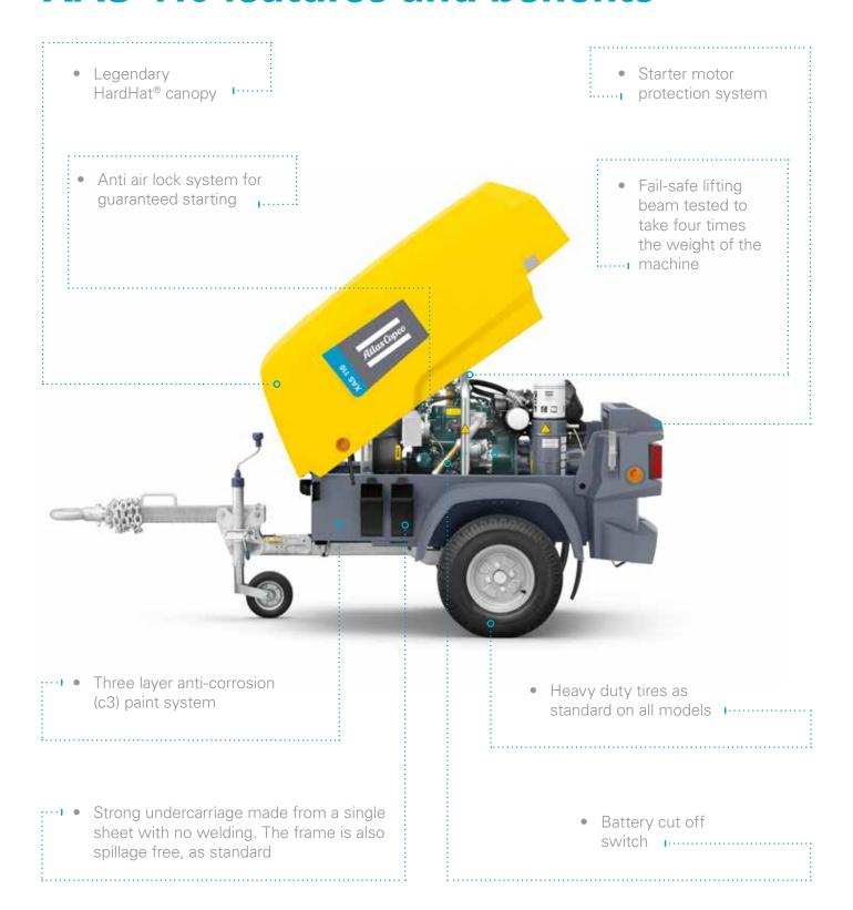
The XAS 110 can power two RTEX breakers and has no need for any exhaust after treatment.
